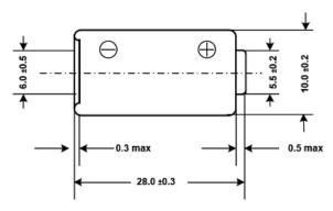
Dimensions are in millimeters and include label.
