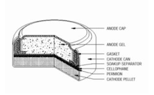
**Cathodes** are a mixture of MnO<sub>2</sub> and conductor.
