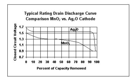
Miniature manganese dioxide batteries typically exhibit an expansion of the cathode on discharge which results in an overall increase in the battery's height. This increase in height is referred to as bulge. While miniature manganese dioxide batteries are designed to minimize bulging, they will typically bulge to a height greater than comparable silver oxide batteries during discharge. Specific bulge data is given on the following individual battery data pages.
