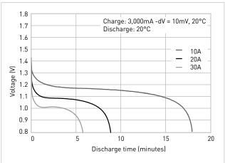
$<sup>^{*1}</sup>$  After charging at 0.1lt for 16 hours, discharging at 0.2lt.
