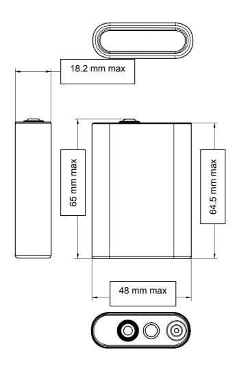
**NOTA :** Following multiple cycling the thickness of the bare cell may go up to 19.0 mm.
