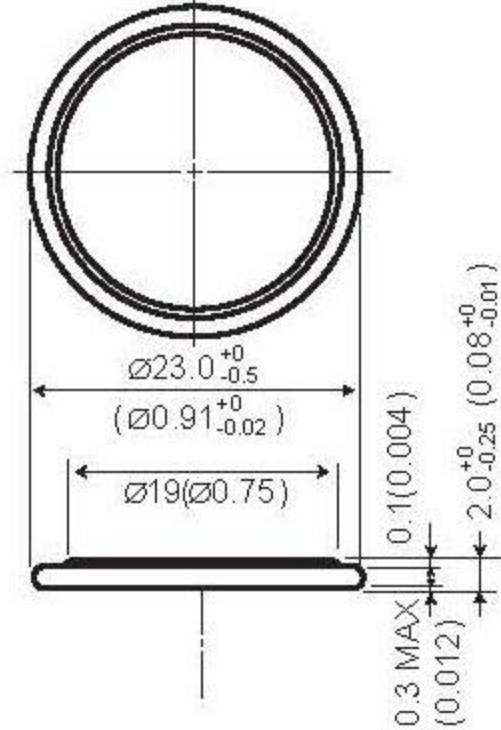
**Note:** This bare cell diagram is for size reference only. Please refer to the tab configurations at the end of this section for available tabs.
