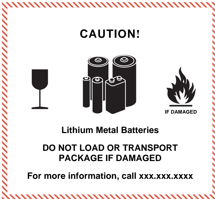
Figure 7.4.H Lithium Battery Label
