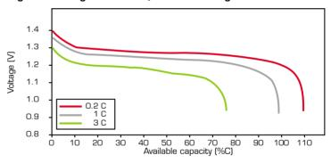
Voltage in discharge at + 20°C (after fast charge 0.1 C x 1.2 hours at + 20°C)
