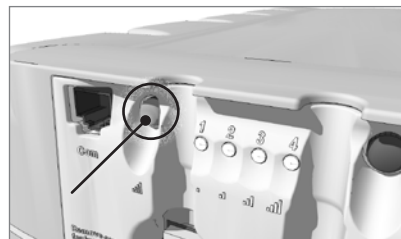
Figure 3 - Checking SOC (State of Charge)
