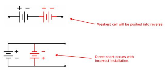
Weaker cells in a parallel configuration will result in either a direct short if cells are installed incorrectly...
